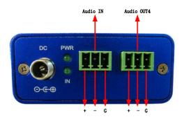
DC IN: 12V 1A. Power socket with fixing lock
