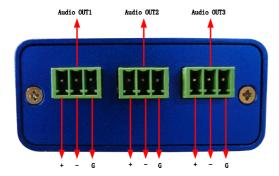
Audio OUT1-3: Three 3pin interfaces are distribution outputs.
